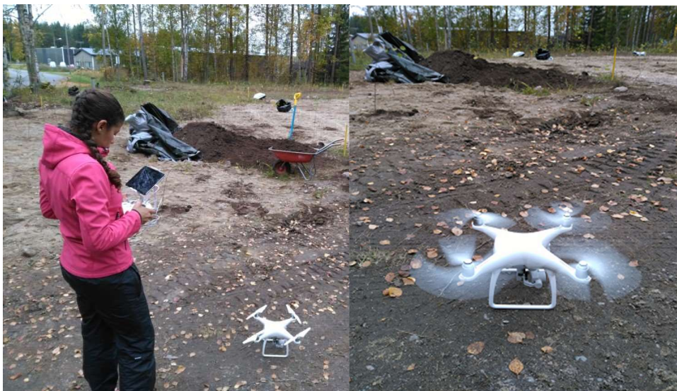
Figure 5.4 a & b. DJI Phantom 4 RPAS equipped with iPad for remote control using specially designed computer program for photographing a preselected area with the mini aircraft
