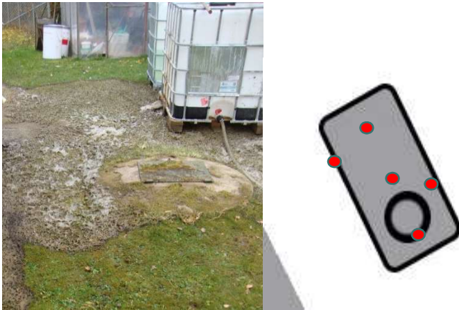
Figure 3.8 a-b. The site after the chemical oxidation treatment (a) and a drawing of the tank with the sampling spots in red (b). Only the results from the three spots on the bottom axis have been used for the surveys, because the other two are higher up the ceiling from where samples could not be withdrawn during all stages of the treatment and also since these concentrations were found to be negligible by comparison.
