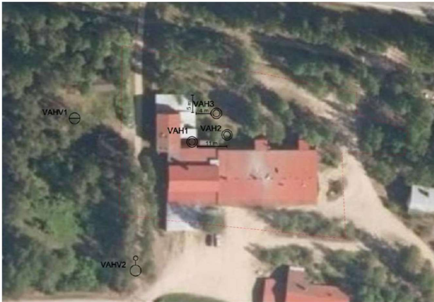
Figure 2.7. The site investigations done by consultant Vahanen Oy with the sampling spots marked.
