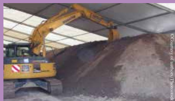
Dynamic aeration cycle using a bucket excavator
