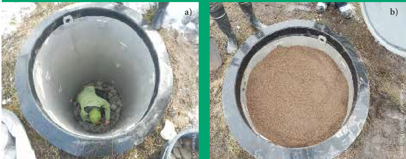
a) Lysimeter and b) soil column for an in situ pilot test at the UHEL lysimeter field station.
