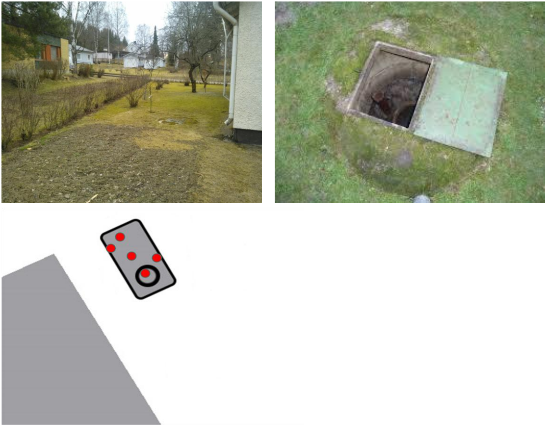
Fig. 1a-c. a-b. Site Janakala c. drawing of the site with sampling/ injection holes drilled into the tank bottom marked by red spots.
