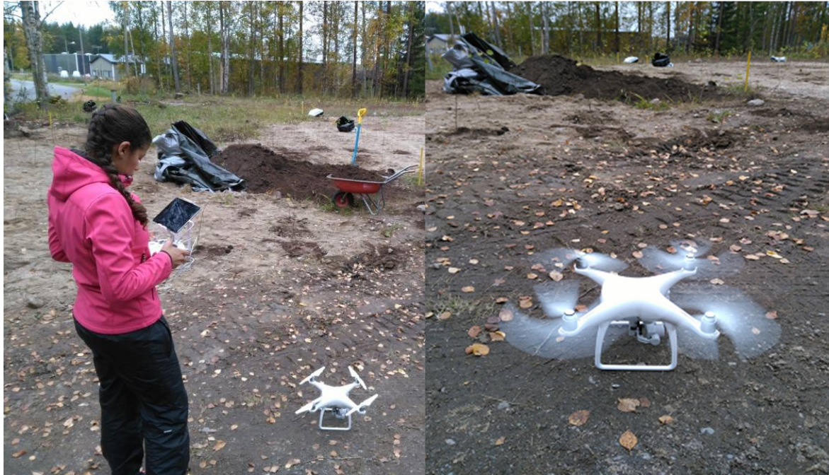
Fig 6.6. DJI Phantom 4 RPAS equipped with iPad for remote control using specially designed computer program for photographing a preselected area with the mini aircraft
