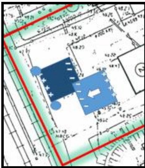
Fig 3.1. The treatment site: the original target area marked in darker blue with the intended electrode rows marked with (+) and (-) symbols. The new chosen site in lighter blue with the suggested anode row marked with (+) and the cathode row with (-). The arrows mark the suspected resulting movement of fluids. The two control drillings outside the treatment area are marked with spots in light blue.
